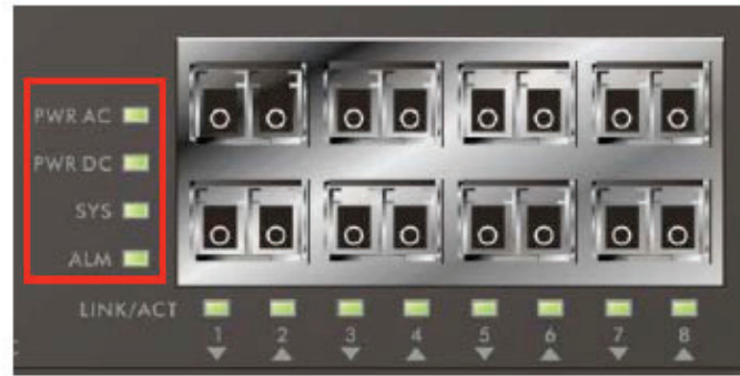
Figure 3-2. System Status LEDs on the front panel.
