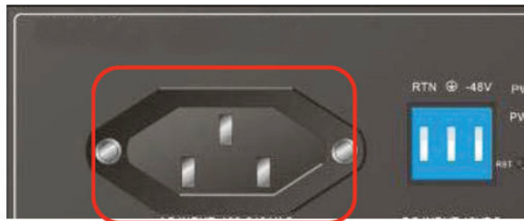
Figure 4-7. Insert the AC power cord into the AC socket to power on this switch.
