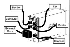
Surge Only Outlets (qty. of 3). These outlets are always **On** (when AC power is available) and are not controlled by the **On/Off** switch. These outlets do not provide power during a power outage. Connect a printer, fax machine or scanner to these
