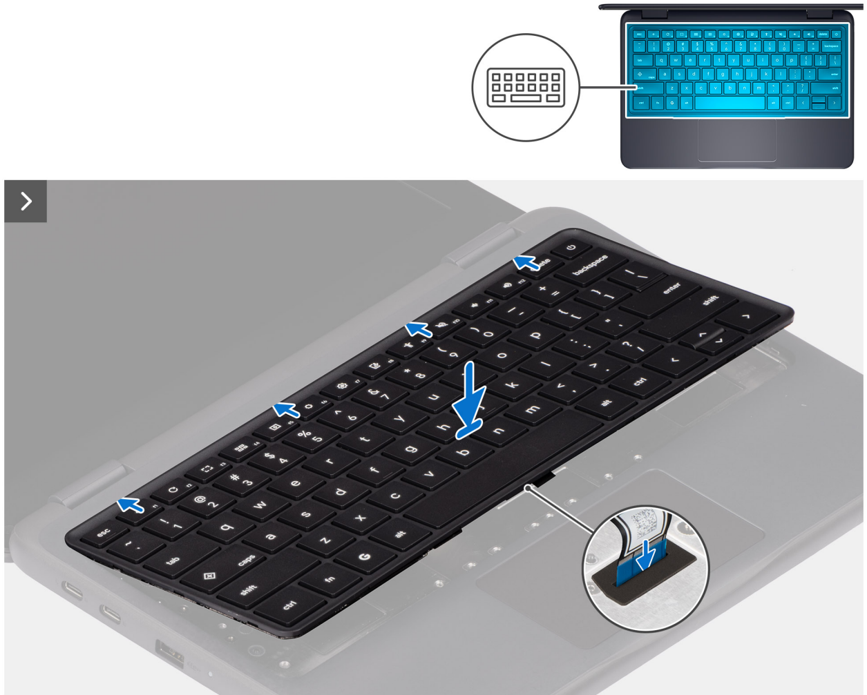
Figure 31. Inserting the keyboard cable through the opening on the palm-rest assembly and placing the keyboard on it
