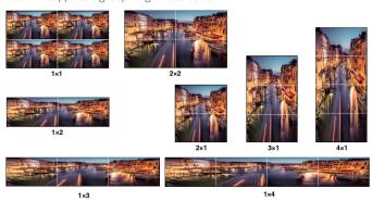
You can set display modes via front-panel buttons, IR remote or RS-232 commands.
