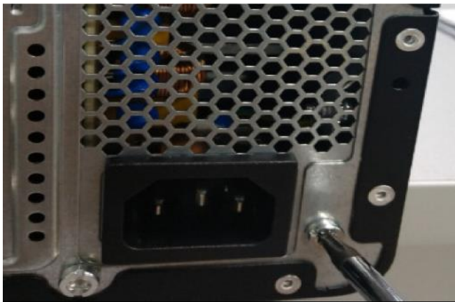
Step 27 Use T-15 screwdriver to release the screws of PSU
