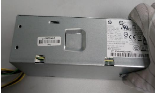
Step 31 Remove the screw and open case
