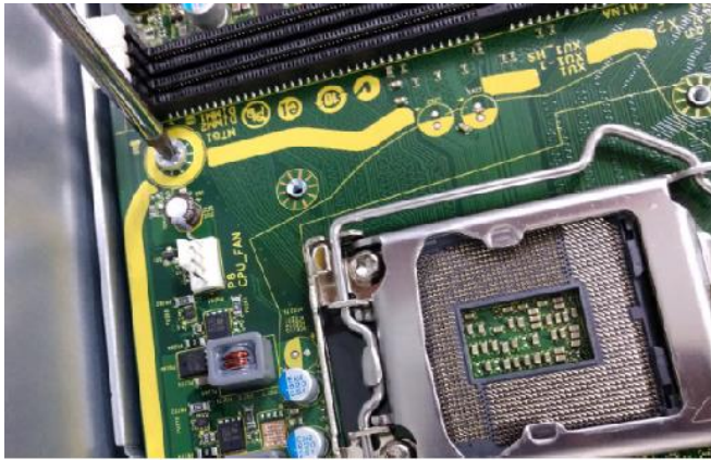
Step 27 Use T-15 screwdriver to release the screws of PSU
