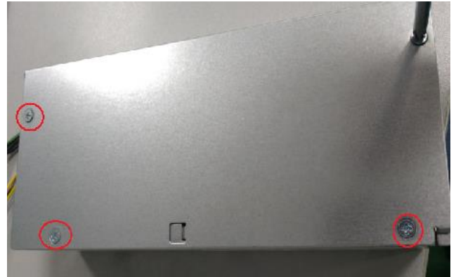
Step 32 Loose screws and remove PCB from case
