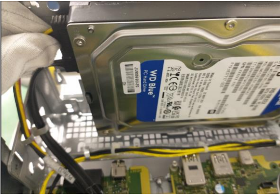
Step9 Remove HDD from Chassis, The PCA of HDD as below:
