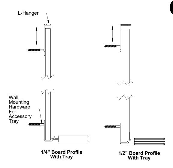
STEP 7: Return board to the wall, secure using the provided #8 x ½" screws.
