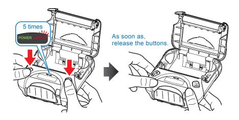
3. After setting a paper, close the printer cover. The set emulation mode is printed out.
