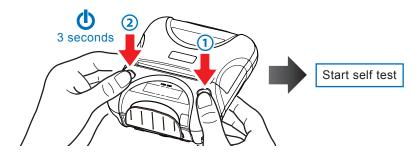
2. After the self test finishes, release the POWER button and the FEED button, and press the POWER and FEED buttons simultaneously within 2 seconds.
