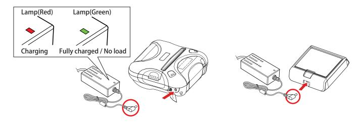
**Note:** When the battery charger is connected to the printer without the battery pack, the printer turns on but cannot print.
