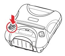
2. To put the printer into Memory Switch Setting mode, press and hold both the POWER & FEED buttons for 3 seconds. After the ERROR LED flashes five (5) times, you can configure the settings. Release the buttons after you surely confirm the LED flashes five (5) times, to get a printer into the setting mode.
