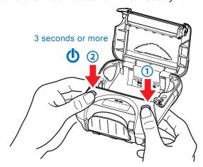
2. After the POWER lamp and ERROR lamp flash alternately, the buzzer sounds and only the ERROR lamp flashes continuously. Then, release the buttons and immediately press and hold the MODE button and the FEED button for three seconds or more, and release the buttons.
