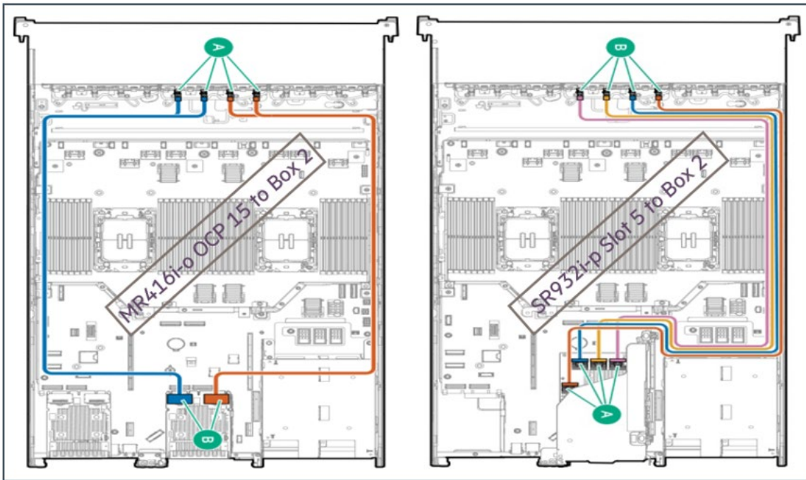
FIGURE 8. 4-socket HPE ProLiant DL560 Gen11 server Box 2 for SAP HANA persistent storage – Controllers to Box 2 connections
