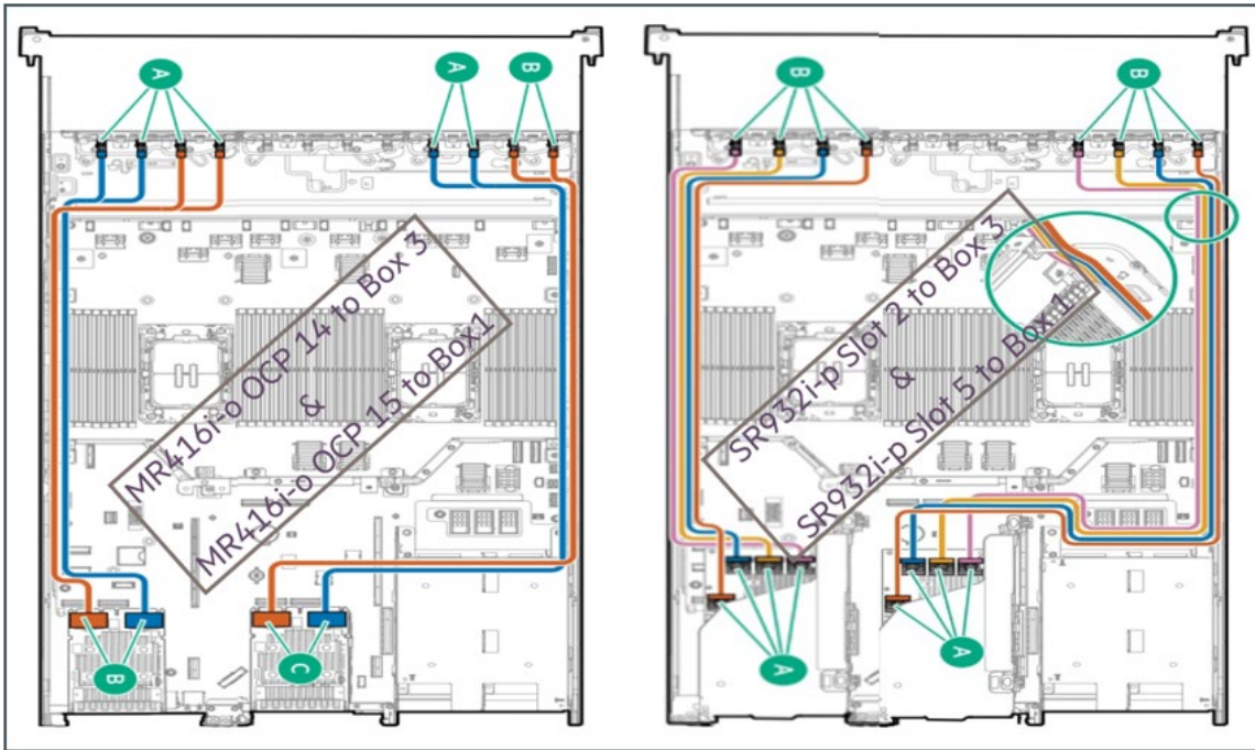
FIGURE 10. 2 or 4-socket HPE ProLiant DL560 Gen11 server Box 3 for SAP HANA persistent storage and Box 1 for Dual-purpose – Controller connections
