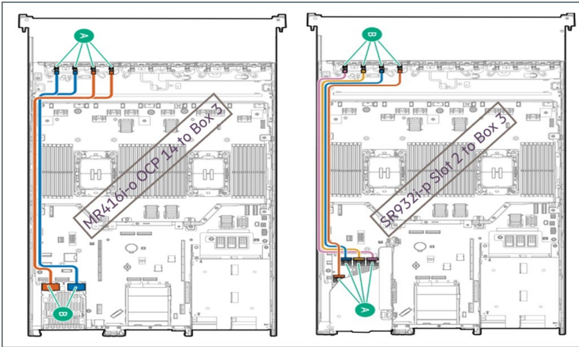
FIGURE 6. 2-socket HPE ProLiant DL560 Gen11 server Box 3 for SAP HANA persistent storage – Controllers to Box 3 connections
