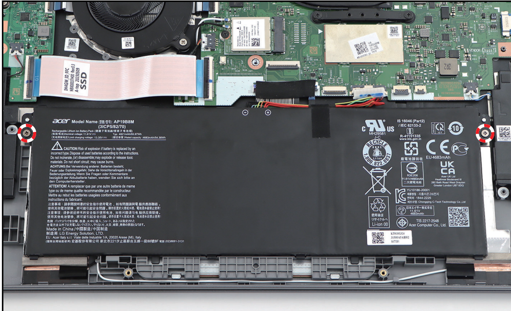
Figure 1-11. Removing the Screws
