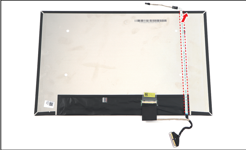
Figure 1-47. Removing the eDP Cable
