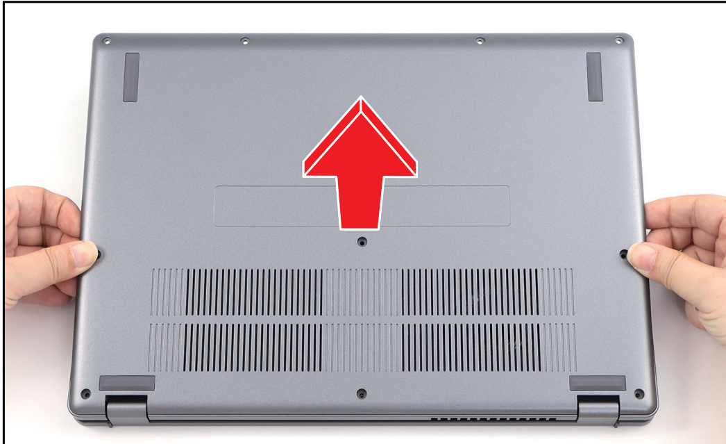
Figure 1-4. Removing the Lower Case
