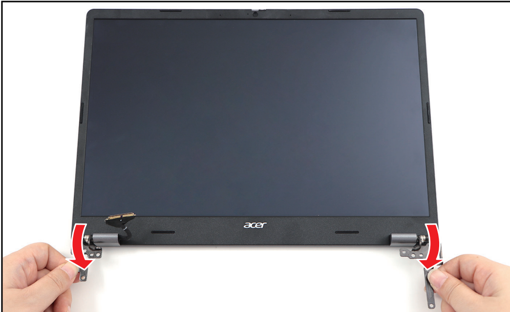
Figure 1-38. Pushing Down the LCD Hinges
