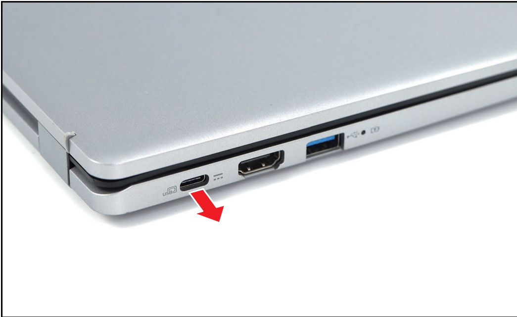
Figure 1-1. Disconnecting the Power Adapter
