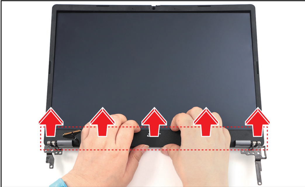
Figure 1-42. Removing the LCD Bezel (4 of 4)
