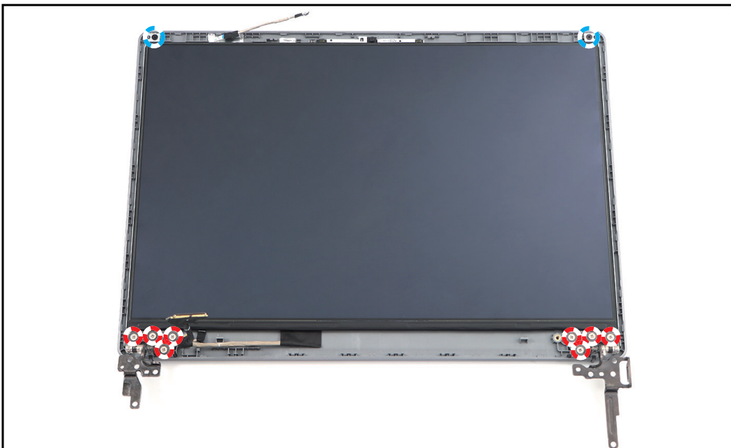
Figure 1-44. Removing the Screws
