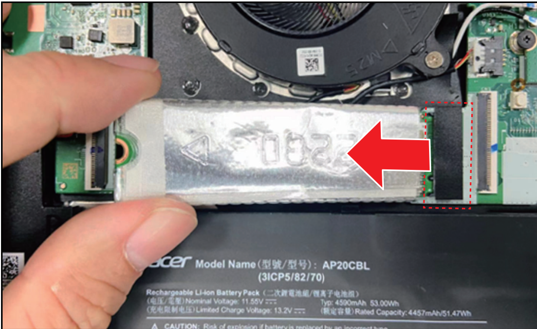
Figure 1-19. Removing the SSD Module
