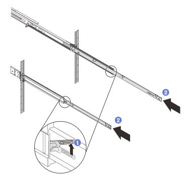
Step 8. Remove the rails from the rack.
