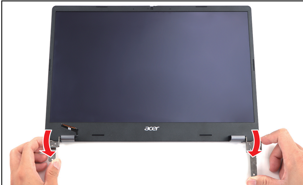
Figure 1-42. Flattening the LCD Hinges
