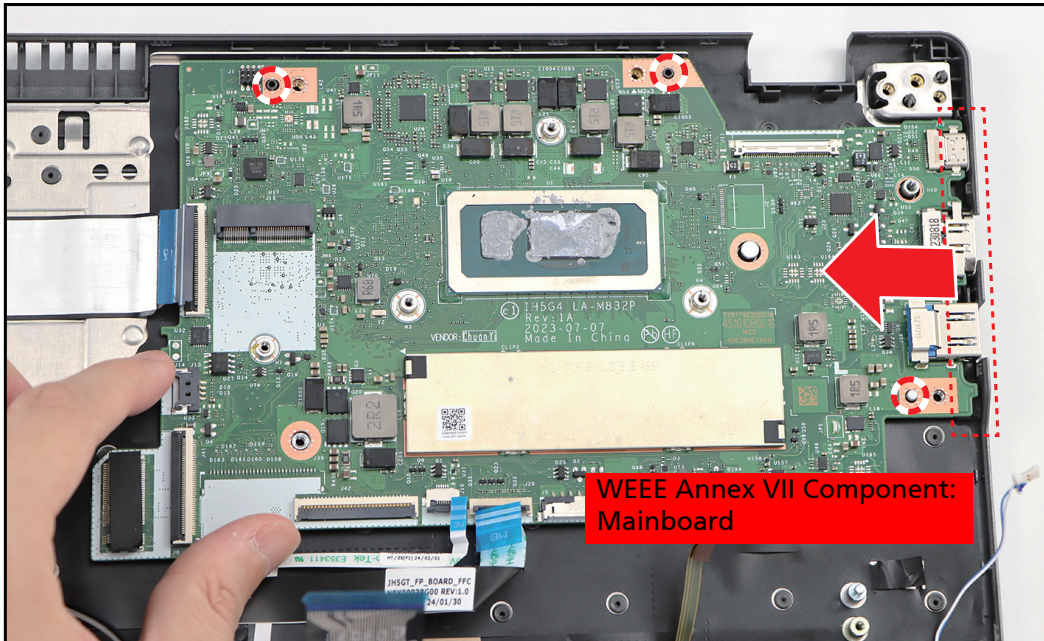
Figure 1-38. Removing the Mainboard
