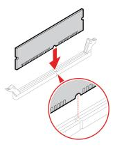
Note: During the installation, ensure that you align the memory module to the slot and press down on both ends until the latches are fully engaged with a click.
