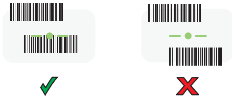
Figure 18 RS6000 Pick List Mode with Multiple Barcodes in Aiming Pattern
