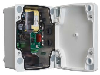
Bosch offers a series of stand-alone power supply units that provide VAC power to AUTODOME 7100i cameras for applications without PoE. Each unit has a cover door that provides IP66/NEMA 4X ingress protection and meets power and electrical safety requirements in extreme environmental conditions. The unique design and the IK10 rating protect the power supply units from vandalism and tampering events.
