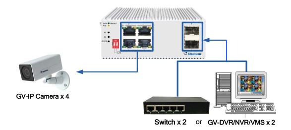
**Note:** To ensure the stability and distance of PoE power transmission, always use 8-core all-copper 0.5 or above national standard cables.
