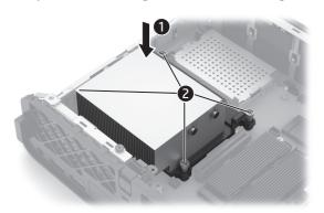
• Connect the fan cable to the system board **1**, lower the fan onto the system board **2**, and secure it with the two screws **3**.
