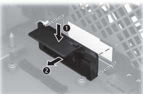
3 Slide the main board adapter into place 1, press down on the connector until it snaps into place 2, and then secure it to the system board 3.
