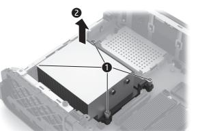
Installing the main board adapter in the HP Z2 Mini G9 computer continued
