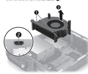
• Remove the four T15 screws in the order shown on the label of the heat sink 1, and then lift the heat sink out of the chassis 2.
