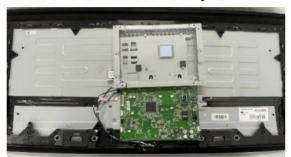
LCD module(together with their casing) is only left after all other parts like electronic units and casing have been removed.
