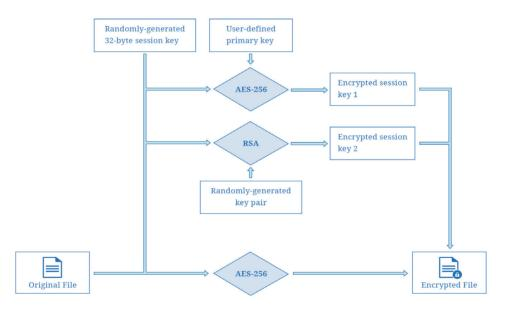
Figure 2: Encryption flow diagram
