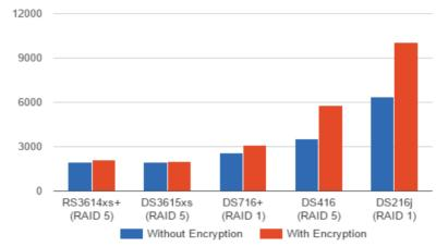
For models with powerful computation power (i.e., RS3614xs+ and DS3615xs), the Disk I/O was the bottleneck, leading to similar results for both the non-encryption and encryption tests.
