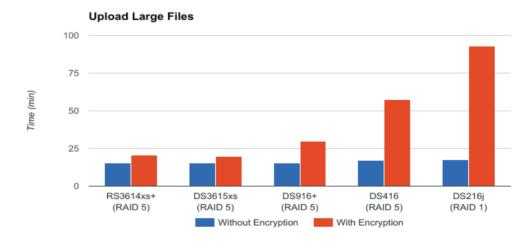
The blue bar shows the results of the cases without data encryption, in which transferring a large file without encryption required about 13.3 minutes. A comparison with the 1Gb Ethernet theoretical values showed that the network I/O was the bottleneck.
