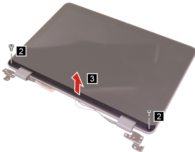
Figure 47. Remove two screws and the LCD bezel
