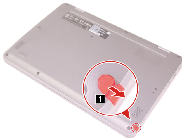
Figure 4. Remove the electronic pen
