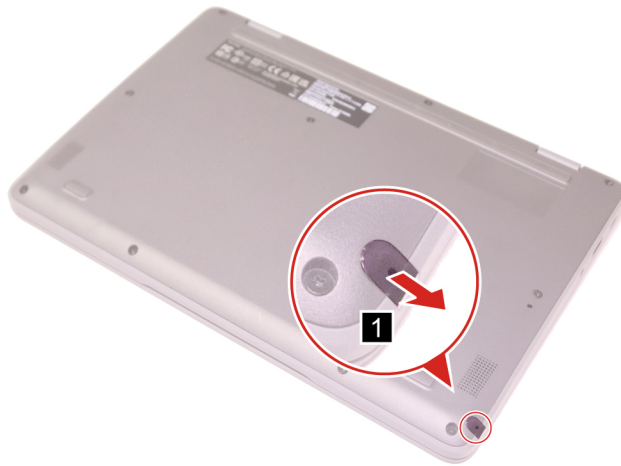
Figure 5. Remove the dummy pen cap
