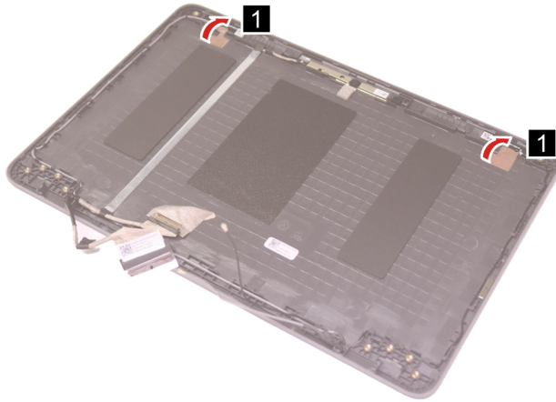
Figure 61. Remove the Wi-Fi antenna tapes
