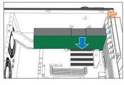
3 Connect the GPU card into the PCle slot on the motherboard. Secure the GPU card assembly to the chassis with four screws.
