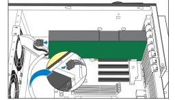
Connect one end of the power cable to the power connector on the GPLI card and the other end of connector on the GPU card and the other end of the power cable to the dedicated connector on the power supply unit (PSU).
