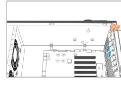
(1) Remove the screw and slide to remove the PCle dummy bracket. Repeat the same procedures to remove another PCIe dummy bracket.
