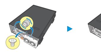
(1) Remove the screw and loosen the thumb screws on the rear of the chassis.
