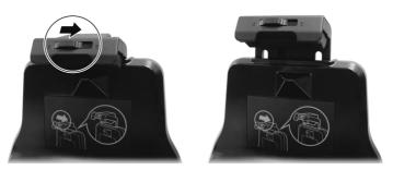
2. Align the connector and place T800 on the dock. Press down the holding clamp until it clicks into place.
