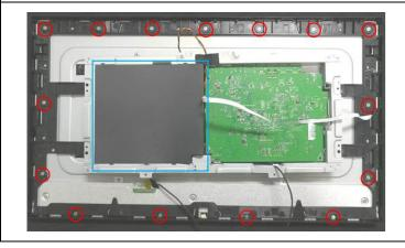
Remove the screw\*8pcs Tool: Screwdriver #2 Disconnect the pins
