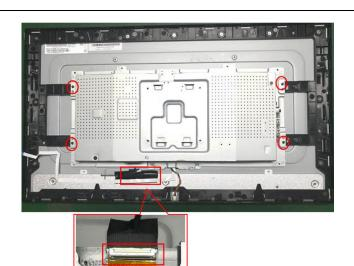
Remove the screw\*15 pcs to separate the panel and the middle frame
