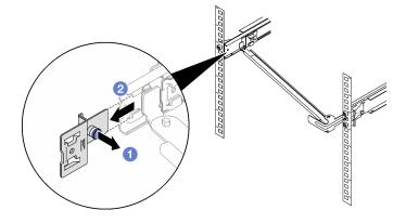
Step 3. Disconnect the stop bracket from the slide rail.
