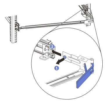
Step 11. Install the CMA mounting bracket into the slide rail.
