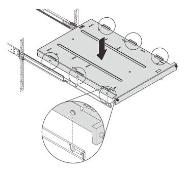
Step 8. Install the CMA support bar.
