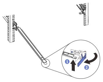
Step 10. Connect the stop bracket to the slide rail.
