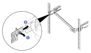
Step 12. Install the CMA into the slide rail.
