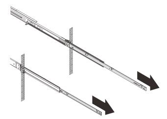
Step 7. Align the nubs on the server rack tray with the holes on the rails as illustrated, and lower the tray until it sits firmly between the two rails and the front nubs click in place.
