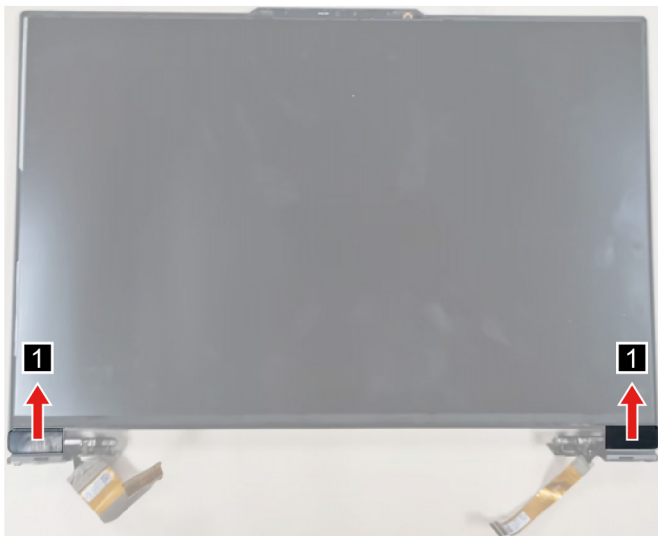
Figure 42. Remove the hinge cover
