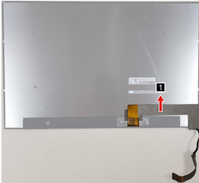
Figure 44. Remove the EDP cable
