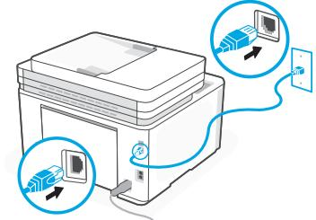
**EN** For wireless setup, do not connect an Ethernet cable. (wireless models only)
