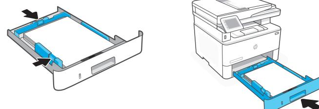
**EN** Load paper and adjust the guides. Open the output tray extender.
