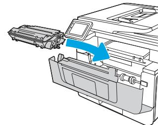
Power off the **original printer** and remove the power cord from the wall outlet, open access door and remove toner cartridge and install toner in your replacement printer along with all other accessories
