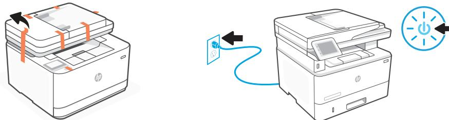
**EN** Remove all tape from the printer. Plug in and power on.
