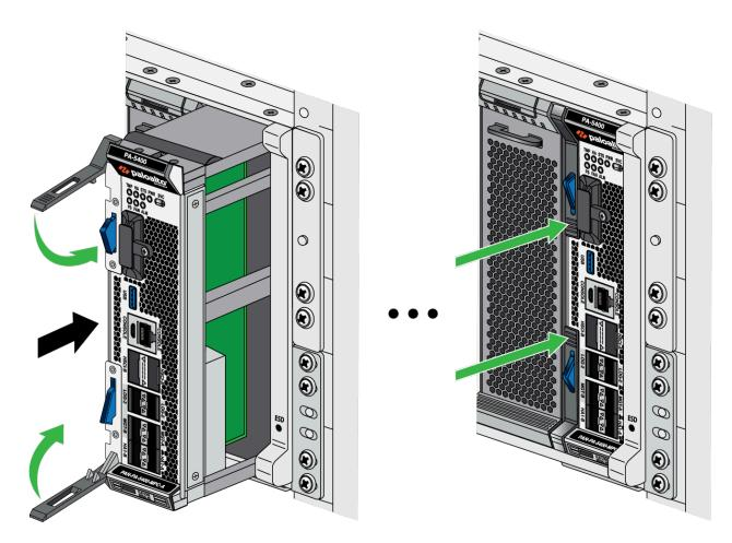
**STEP 3** Rotate the card and align it with the front of the appliance so that the Palo Alto Networks logo is readable at the top of the card. Gently push the NC into slot 1 until the card reaches the end of the slot.
