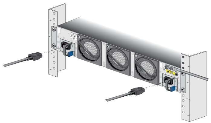
2. Secure the power cords to the power inlets using the velcro straps.
