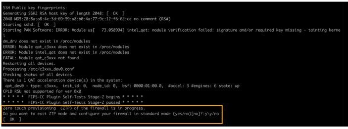
If you miss the above CLI prompt, you can also change your boot mode using the web interface. Go to the firewall login screen at any point before or during the startup process. A prompt will ask if you wish to continue booting in ZTP mode or if you would like to switch to standard mode. Select **Standard Mode** and the firewall will begin rebooting in standard mode.
