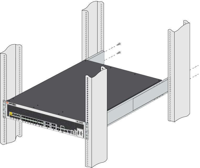
two screws for each bracket (#10-32 x 3/4" or #12-24 x 1/2" screws) and torque each screw to 25 in-lbs.
