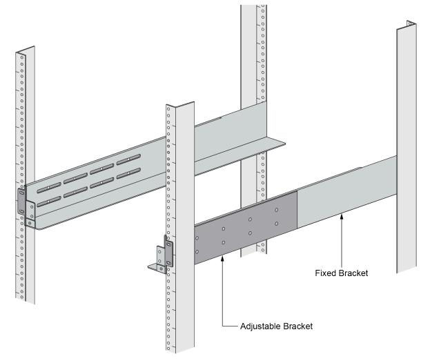
**STEP 4** Adjust the brackets to fit the depth of the equipment frame, then secure the brackets to the equipment frame with mounting screws (not provided) compatible with your equipment frame. Tighten the screws to their recommended torque value.
