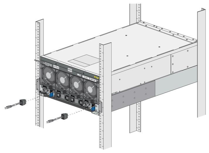
**2.** Secure the power cords to the power inlets using the power cord retainer clips.
