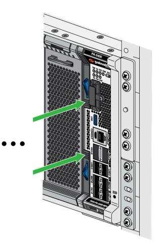
**STEP 3** Rotate the card and align it with the front of the appliance so that the Palo Alto Networks logo is readable at the top of the card. Gently push the DPC into slot 3 until the card reaches the end of the slot.
