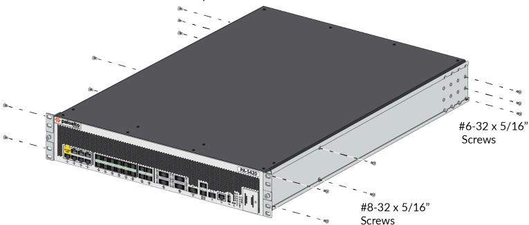
**STEP 3** With help from another person, hold the firewall in the rack and secure the fixed rack mount brackets to the front rack-posts using four screws for each bracket. Use the appropriate
