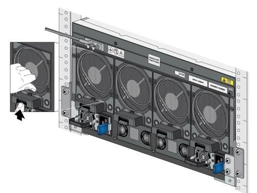
**STEP 5** While still gripping the fan assembly handle, gently pull the fan assembly out of its slot.
