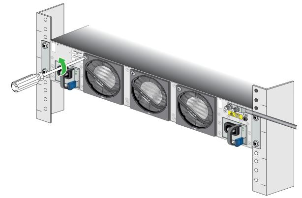
**STEP 5** While gripping the fan assembly handle, gently pull the fan assembly out of its slot.
