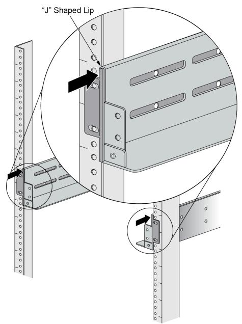
**STEP 3** Position the bottom edges of the fixed and adjustable brackets to the bottom of the 5 RU rack space reserved for the PA-5450. Align the slotted holes of the fixed mounting bracket
