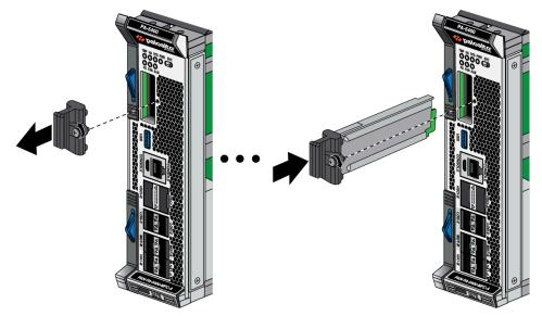
**STEP 4** Once the logging drive is fully seated, tighten the retainer screw to 4 in-lbs.
