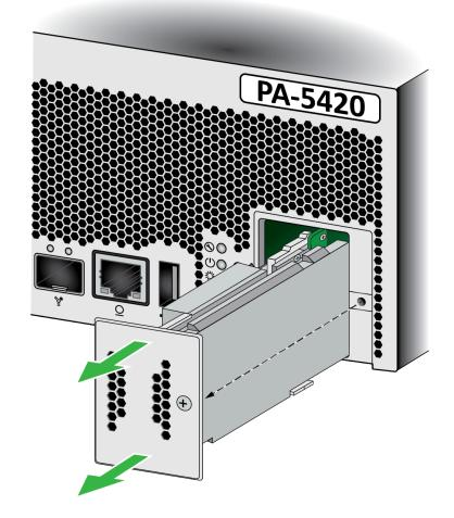
**STEP 7** Remove the replacement drive from the packaging, determine the drive model, and place it on an antistatic surface. Then compare this model number with the model number of the failed drive to determine which replacement procedure to use in Step 9.
