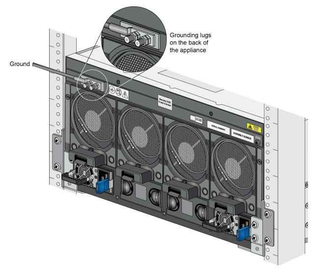
**STEP 6** | Crimp a 6-AWG wire to the provided grounding lug and connect the other end to your earth ground point.
