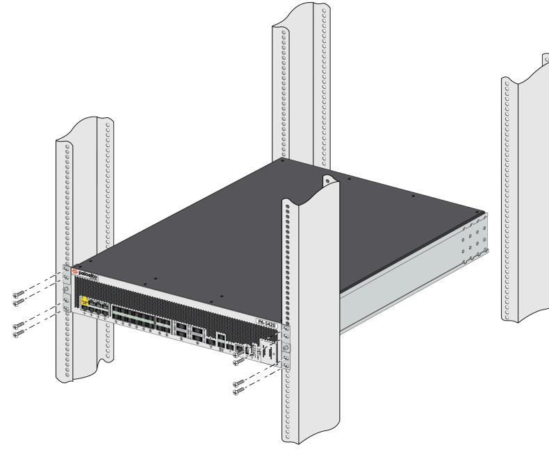
**STEP 4** | Slide one adjustable rack mount bracket into each of the two previously installed fixed rack mount bracket. Secure the two adjustable rack mount brackets to the back rack-posts using
