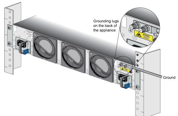
**STEP 5** | Crimp a 6-AWG wire to the provided grounding lug and connect the other end to your earth ground point.
