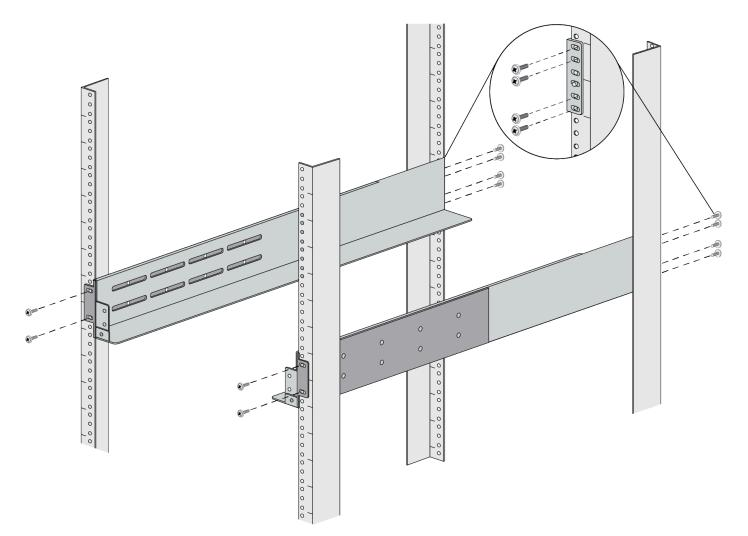
**STEP 5** Use the provided 6-32 x 5/16 flathead screws to secure the adjustable bracket to the fixed bracket. A minimum of 6 screws are required for each side.
