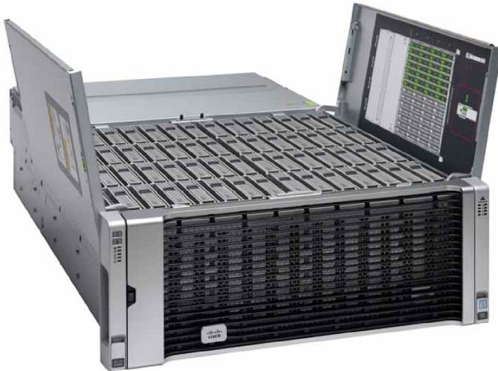
Figure 1. Cisco UCS S3260 Storage Server
