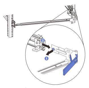
Step 4. Remove the CMA stop bracket.
