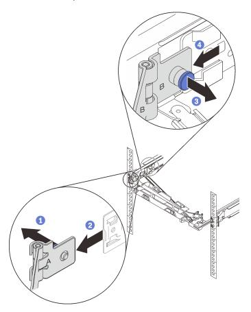
Step 2. Remove the CMA mounting bracket from the slide rail.
