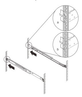
Step 3. Unlock the slide rail lock.
