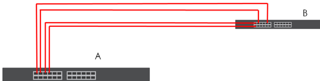
Figure 107 Trunking Example – Physical Connections
