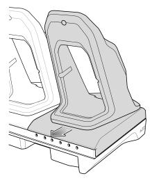
7. Using a Phillips screwdriver, secure the new ethernet cup to cradle with screw.
