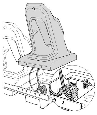
5. Connect the new ethernet cup cables to the connectors.
