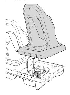
6. Align the new ethernet cup with the cradle and slide the ethernet cup back.
