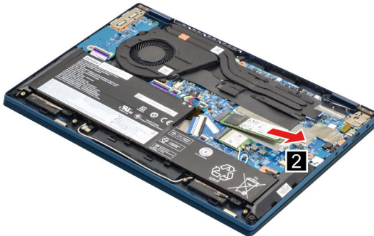
Figure 9. Remove the SSD
