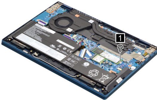
Figure 8. Remove one screw
