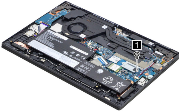
Figure 41. Remove one screw
