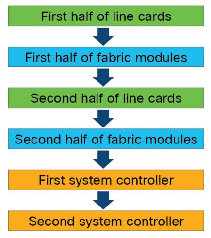
The steps for the parallel upgrade process on Cisco Nexus 9500 Series switches are:
