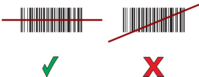
Figure 11 Linear Scanner Aiming Pattern
