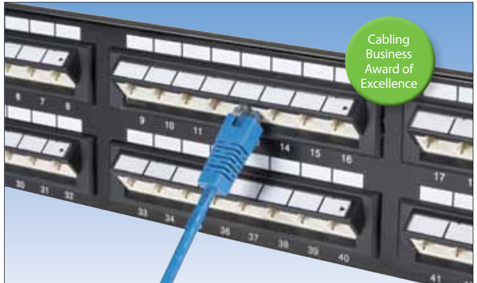
45° angled ports allow for patch cables to drape down, freeing up to 4" of cabinet depth. You'll also save time and money by eliminating horizontal cable managers in front of the panel. Shown: JPM648-45ANG
