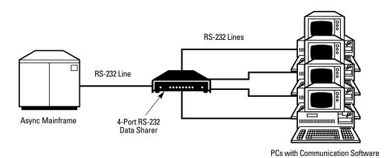
Asynchronous application—an RS-232 Data Sharer providing four PCs with access to an async host.
