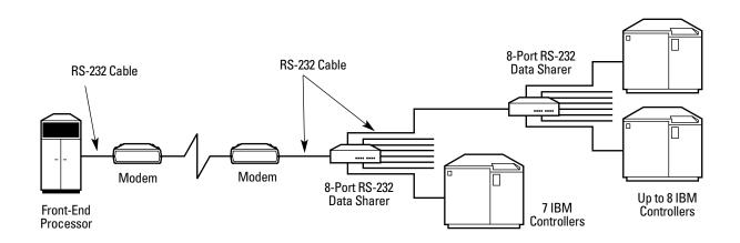
Connect up to 15 remote controllers to a front-end processor by cascading RS-232 Data Sharers.
