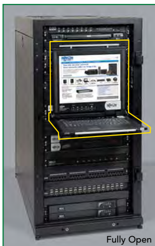
Console KVM Switches fold like a laptop and slide into a 1U rack drawer.
