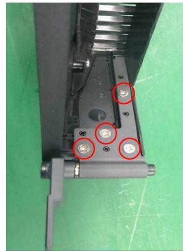
Remove the COVER\_ANTENNA from BEZEL.
