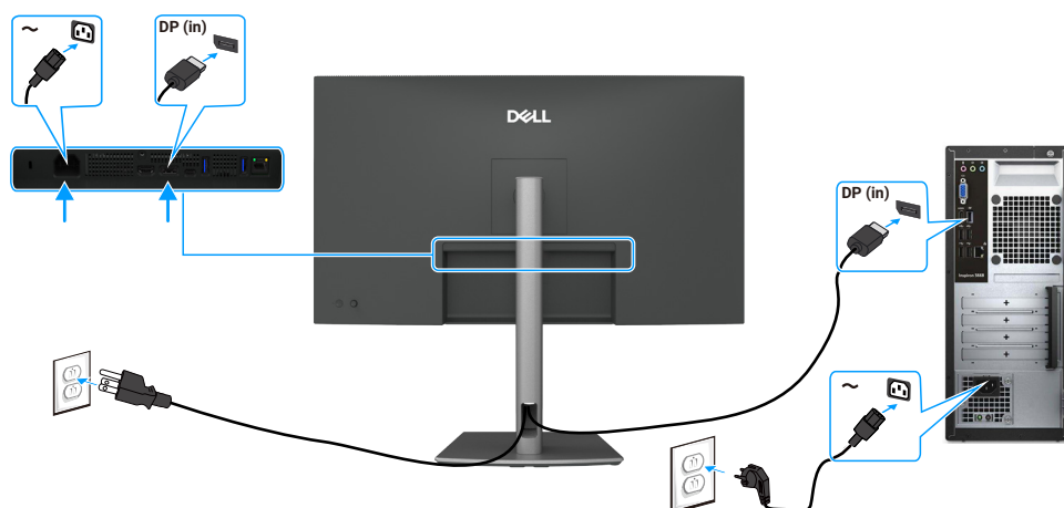
Figure 9. Connecting the DisplayPort cable
