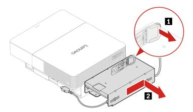
**Note:** Hold the latch in step **1** when removing the power adapter cage.
