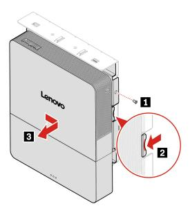
**Note:** Hold the latch in step **2** when removing the top bracket.
