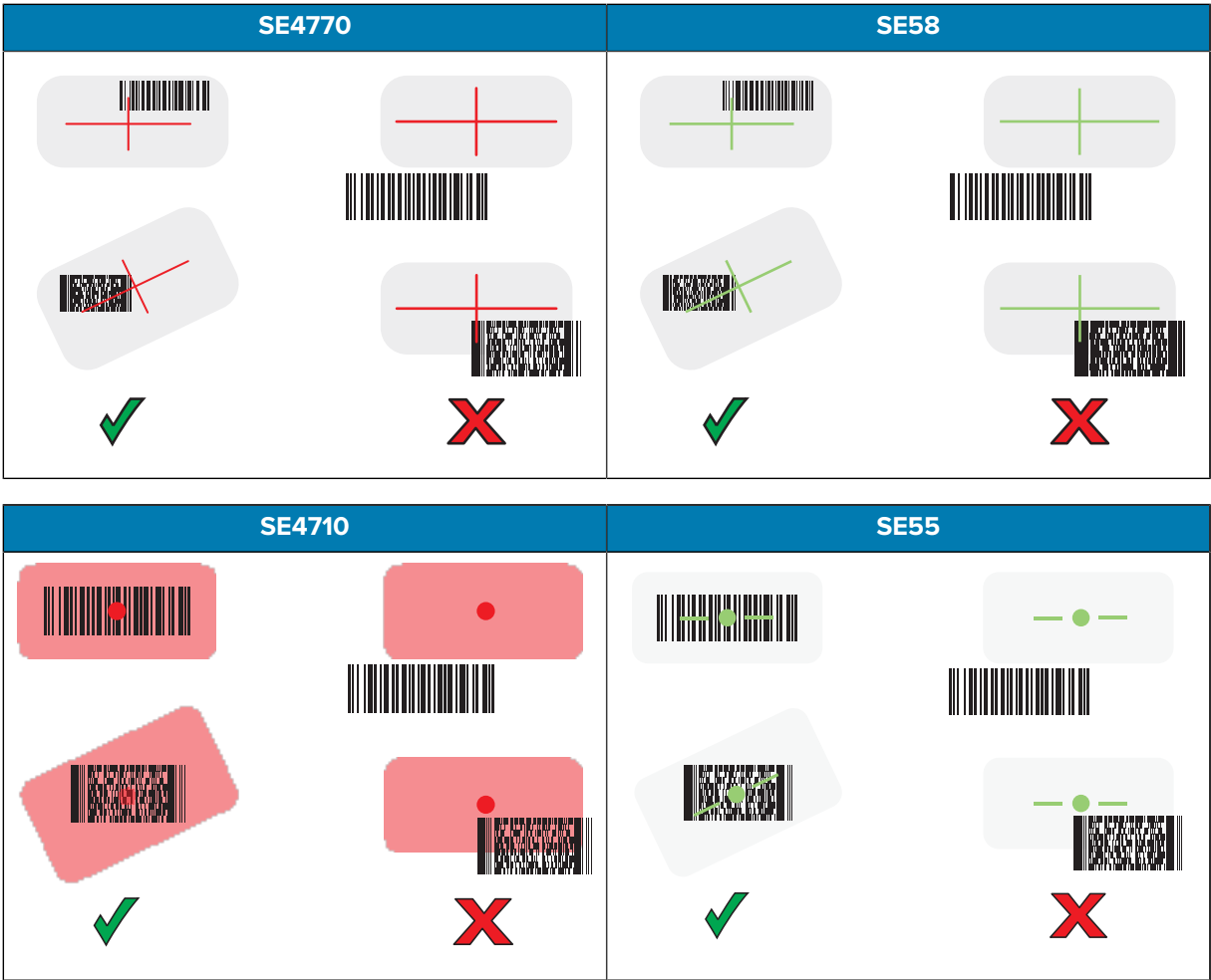
Figure 17 Picklist Mode with Multiple Barcodes in Aiming Pattern
