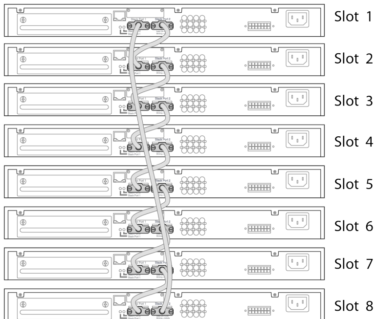
Figure 30: SummitStack Cable Connections Using Eight Switches with Integrated SummitStack Ports
