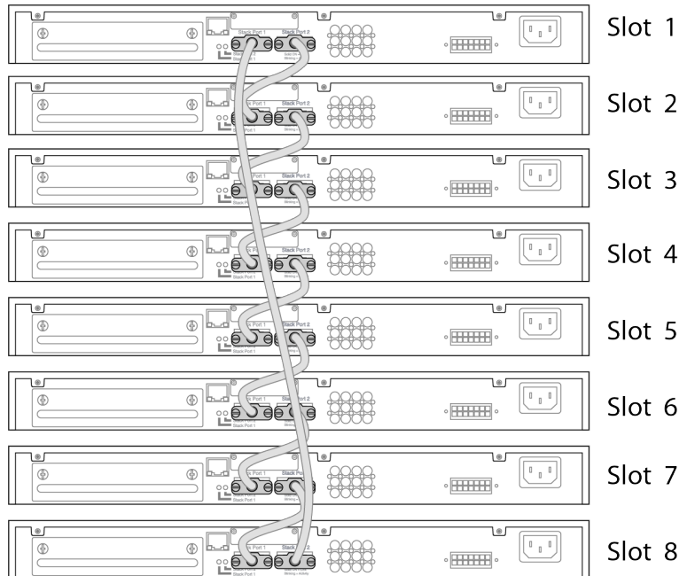
Figure 28: SummitStack Cable Connections Using Eight Switches with Integrated SummitStack Ports
