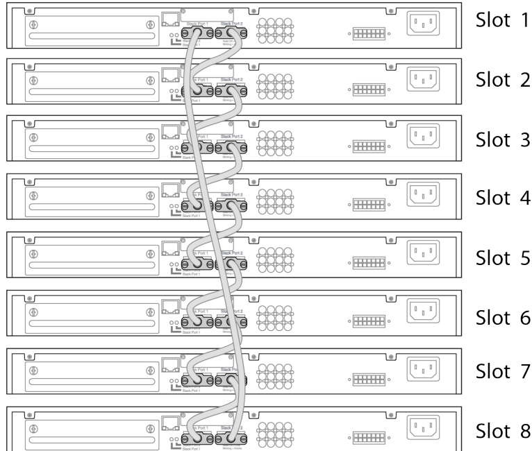
Figure 43: SummitStack Cable Connections Using Eight Switches with Integrated SummitStack Ports
