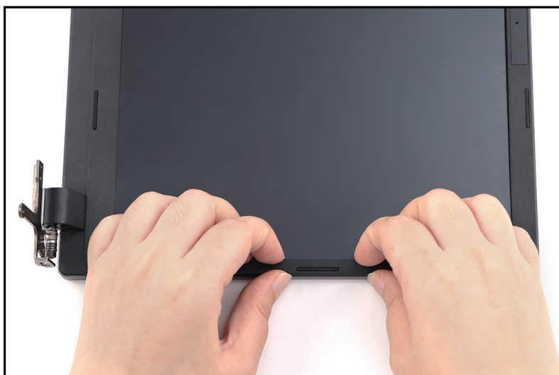
Figure 1-50. LCD Bezel Removal
