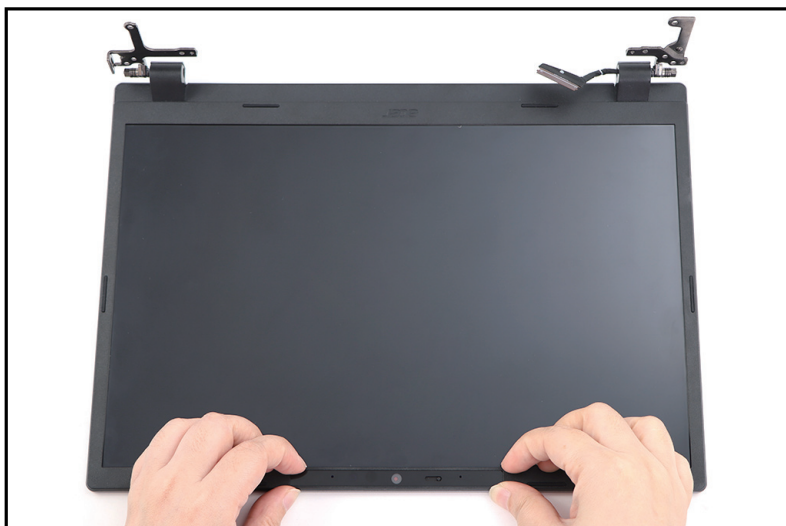
Figure 1-49. LCD Bezel Removal
