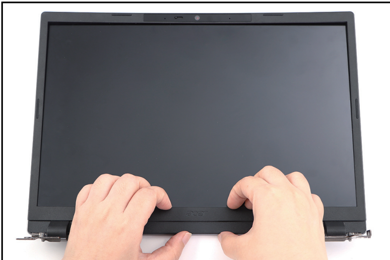
Figure 1-52. LCD Bezel Removal
