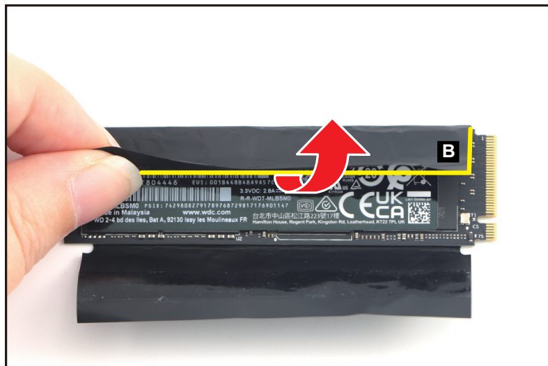
Figure 1-14. SSD Module Removal
