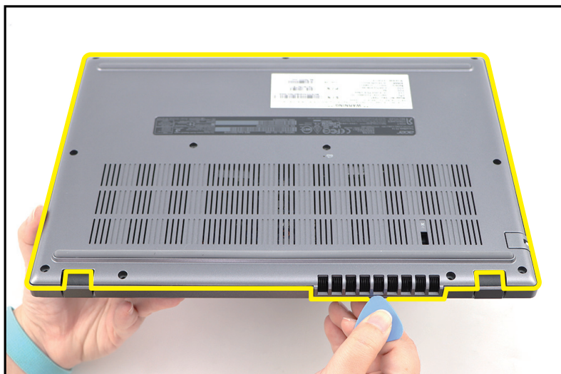
Figure 1-4. Base Cover Removal
