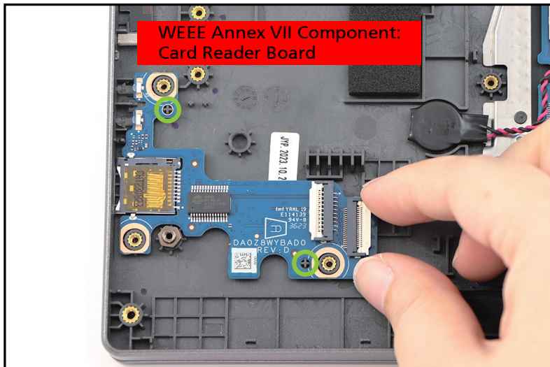
Figure 1-38. Card Reader Board Removal
