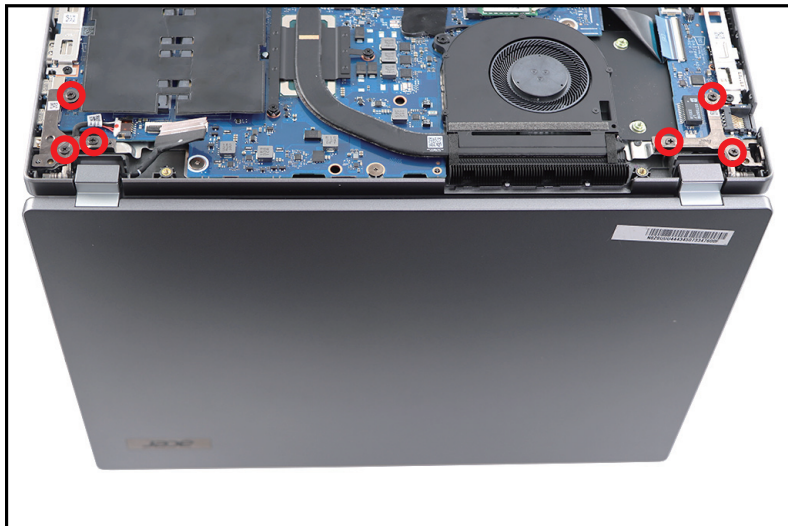
Figure 1-26. LCD Module Removal
