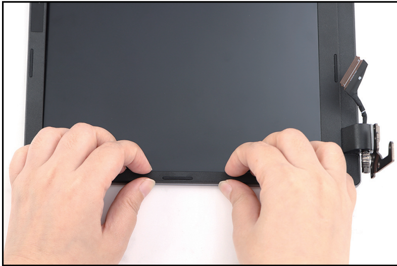
Figure 1-51. LCD Bezel Removal
