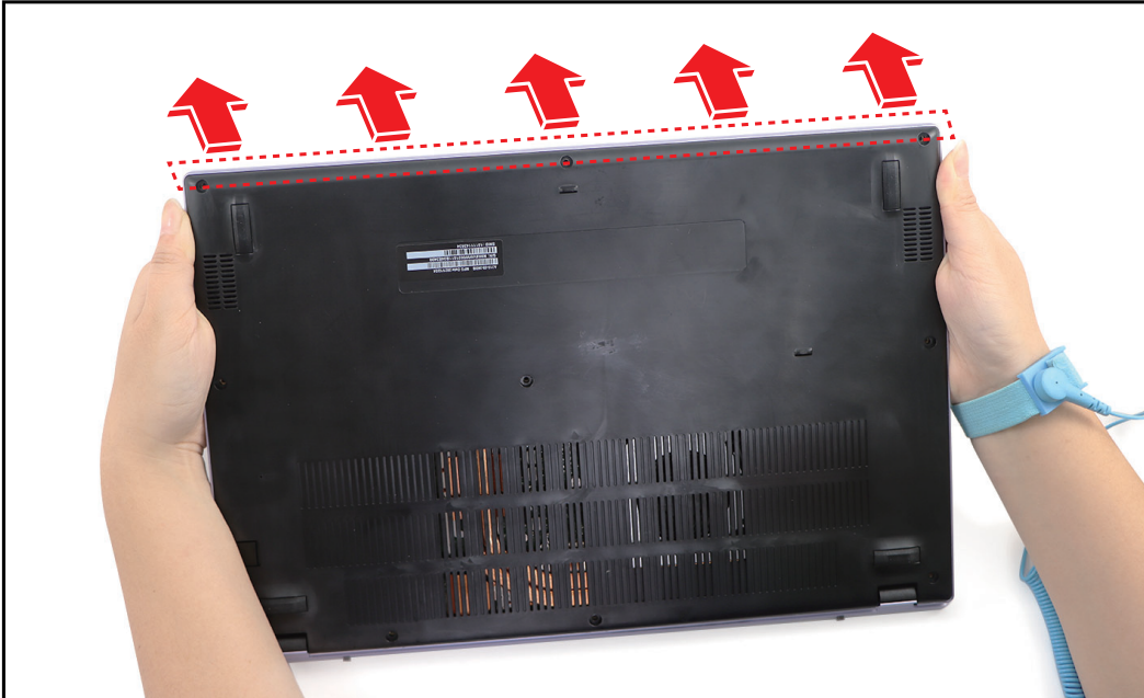
Figure 1-3. Releasing the Lower Case
