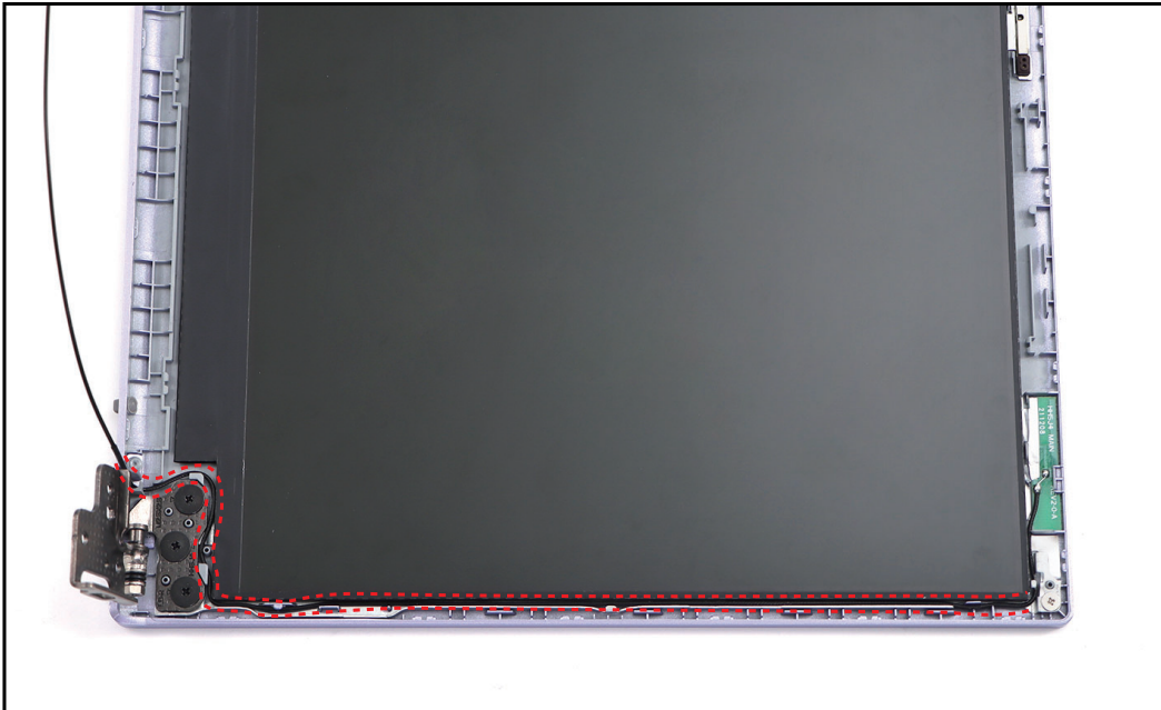
Figure 1-48. Unrouting the Main Antenna Cable
