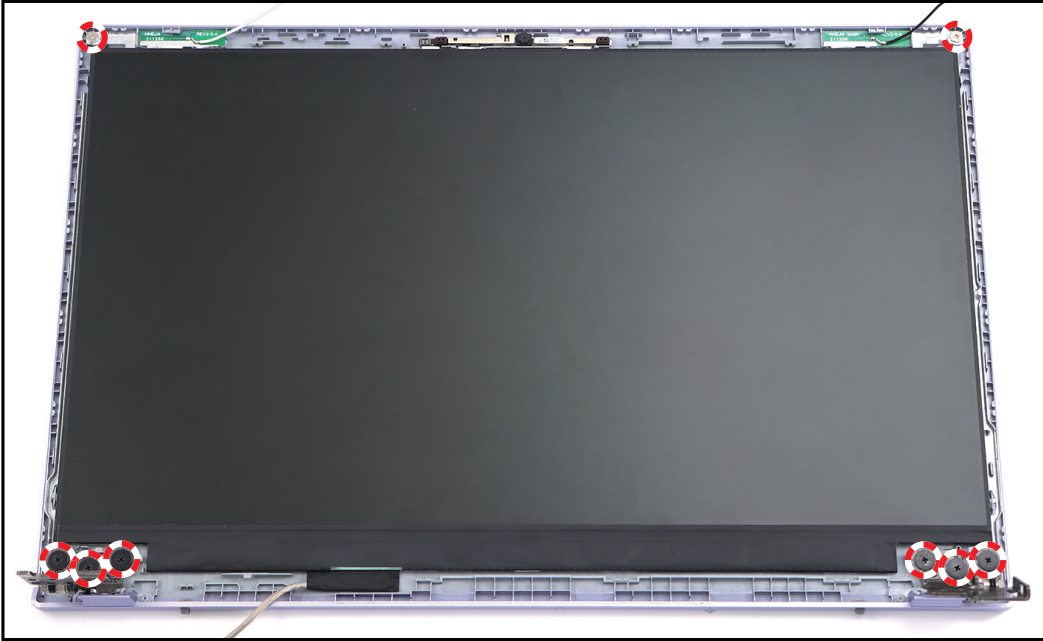
Figure 1-49. Removing the Screws
