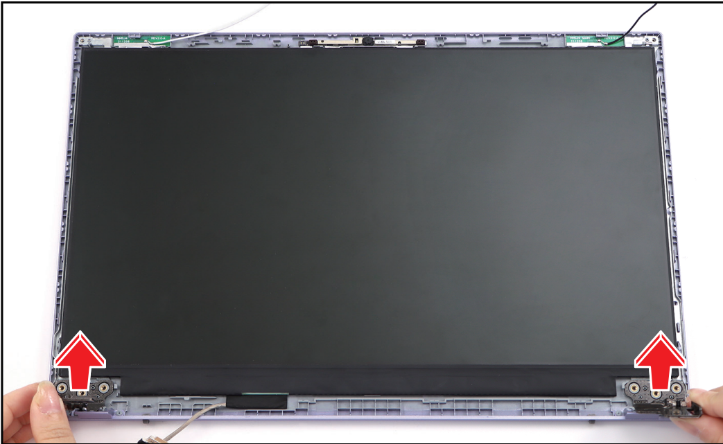
Figure 1-50. Removing the LCD Hinges
