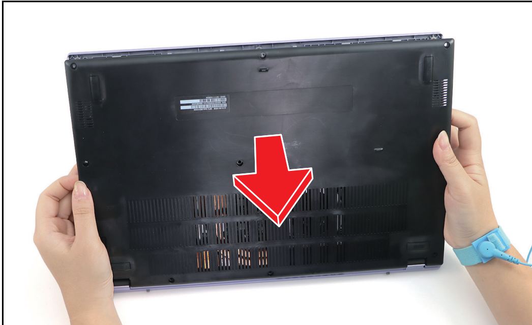
Figure 1-4. Removing the Lower Case
