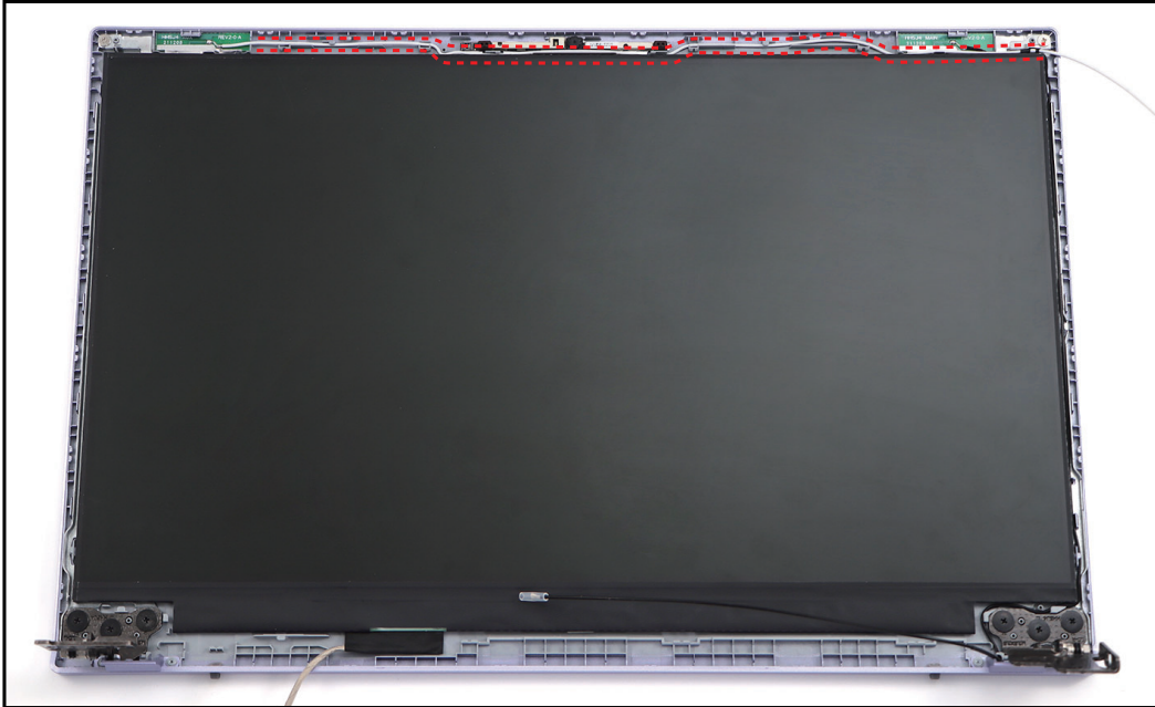
Figure 1-47. Unrouting the Auxiliary Antenna Cable (2 of 2)
