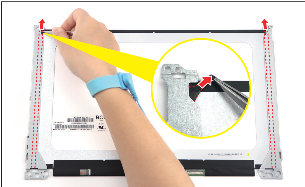
Figure 1-55. Detaching the Double-sided Mounting Tapes
