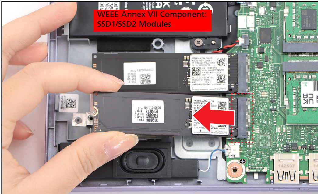
Figure 1-10. Removing the SSD Module
