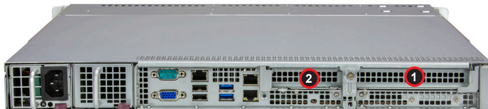
Figure 3-7. Expansion Card Slots in the Chassis
