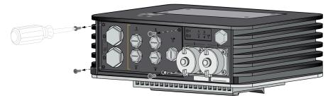
2. On the removed panel, unscrew the stopping plug that lines up with the DC power input you are connecting to.
