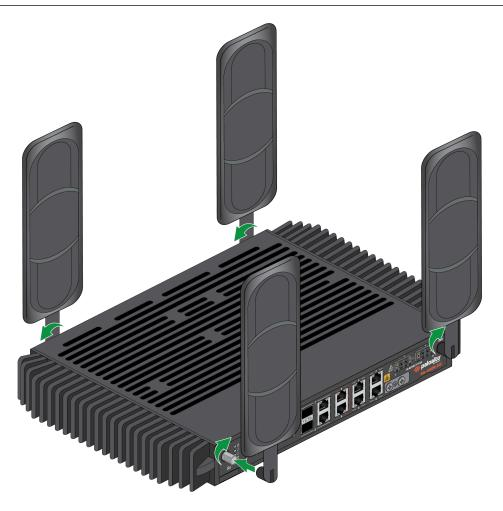
**STEP 2** Adjust the antenna orientation to receive the optimal signal strength in your environment.
