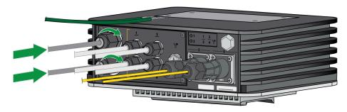
STEP 9 | Power on the DC power source to power on the firewall. The firewall powers on and the power LED turns green.
