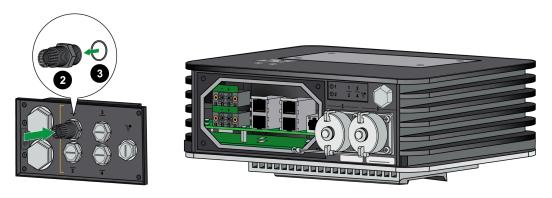
STEP 5 | Thread the Ethernet cable through the end cap. This is used to secure the cable gland once the panel is reattached at the end of the procedure. Feed the Ethernet cable through the
