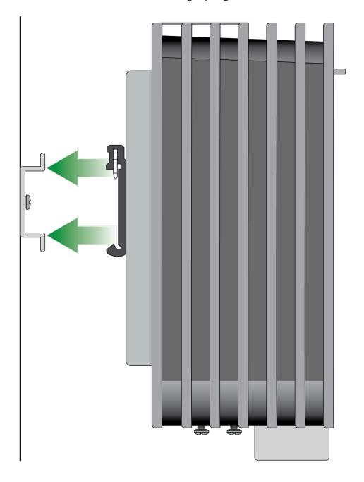
STEP 2 | Using slight downward pressure, attach the firewall onto the DIN rail so that the two metal clips lock into place.
