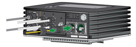
STEP 5 | Push the connector up to the the SFP port and turn the connector clockwise until there is a click. Make sure that the connector is securely locked in place.
