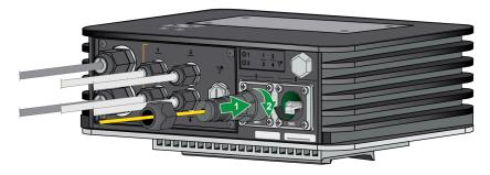
STEP 6 | Screw the end cap into the seal and tighten it until the end cap is securely fastened.
