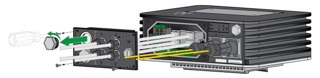
3. Unpack the power cable glands. There are four items — an end cap, panel connector, lock nut, and seal.
