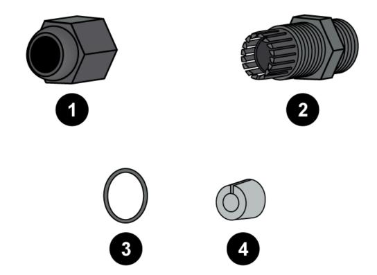
4. Loop the seal onto the shorter end of the panel connector. Make sure to push the seal until it is flush against the nut. Screw the shorter end of the panel connector into the hole that corresponds to the DC power input being connected. Make sure that the connector is secure.
