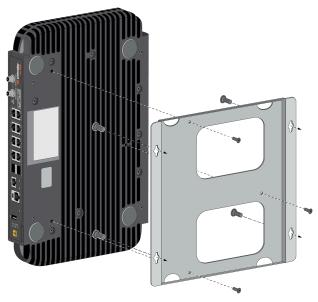
STEP 3 | Attach the wall mount to the wall using four screws that are appropriate for your wall. Sheet metal and drywall inserts are included with the wall mount kit.
