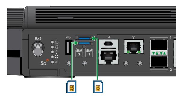
STEP 3 After inserting the SIM, place the SIM cover back onto the device and fasten the two screws.
