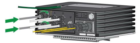
**STEP 9** Power on the DC power source to power on the firewall. The firewall powers on and the power LED turns green.
