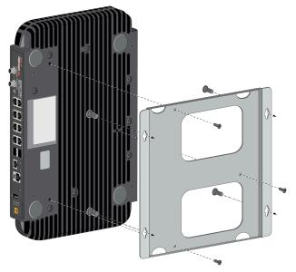
**STEP 3** Attach the wall mount to the wall using four screws that are appropriate for your wall. Sheet metal and drywall inserts are included with the wall mount kit.
