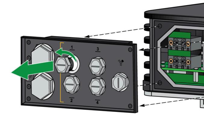
**STEP 3** Unpack the Ethernet cable glands. There are five items – an end cap, panel connector, lock nut, seal, and grommet.
