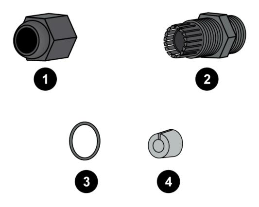
**STEP 4** Install the seal onto the shorter end of the panel connector. Make sure to push the seal until it is flush against the nut. Screw the shorter end of the panel connector into the hole that corresponds to the Ethernet port being connected. Make sure that the connector is secure by torquing to 1.5 Nm.
