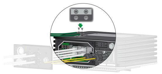
**STEP 4** | (PA-410R and PA-410R-5G only) Thread the power cable through the assigned hole in the bottom panel.
