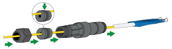
**STEP 4** Connect the fiber cable to the installed transceiver. Move the three cable gland components towards the firewall. Push the seal into the connector.
