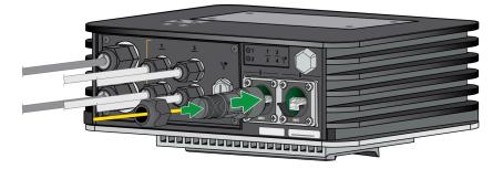
**STEP 5** | Push the connector up to the the SFP port and turn the connector clockwise until there is a click. Make sure that the connector is securely locked in place.
