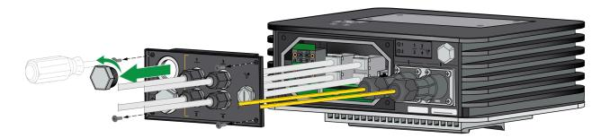
3. Unpack the power cable glands. There are four items — an end cap, panel connector, lock nut, and seal.
