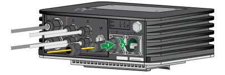
**STEP 6** Screw the end cap into the seal and tighten it until the end cap is securely fastened.
