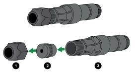
**STEP 3** | Thread the fiber cable through the end cap. Unlatch the seal and fit the cable into it, then close the seal latch. Thread the fiber cable through the connector so that the three components are in the order pictured.
