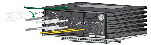
3. Push the end caps along each Ethernet and power cable until the end caps reach their respective panel connector. Screw the end caps onto each panel connector, making sure that it is tight and secure.
