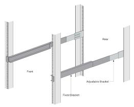
**STEP 2** Align the bottom edge of the mounting rails to the bottom of the 1 RU (1.5 RU if there is another device above) reserved for your firewall. Align the slotted holes in the adjustable mounting bracket to the holes on the rear of the equipment frame.
