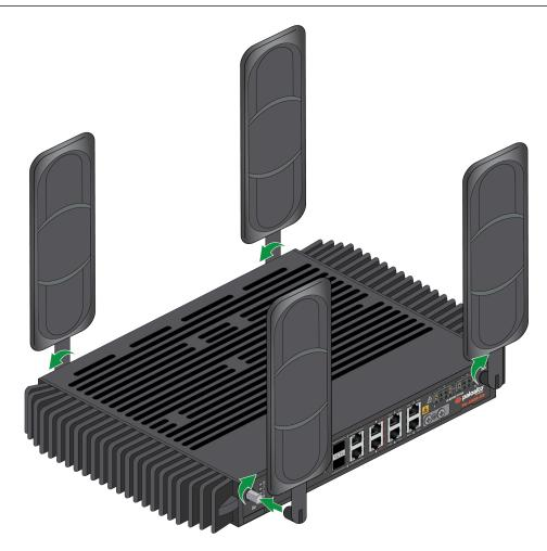
**STEP 2** | (PA-410R-5G only) Fold the antennas at a 90 degree angle so that the device can be appropriately installed on a wall or DIN rail. While viewing the back panel of the device,
