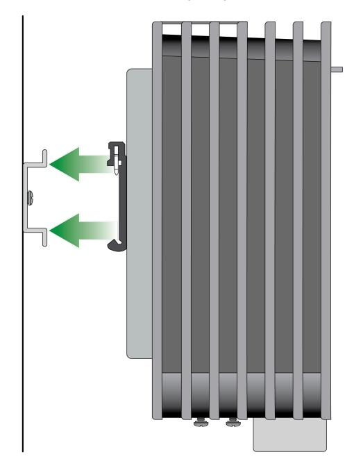
**STEP 2** Using slight downward pressure, attach the firewall onto the DIN rail so that the two metal clips lock into place.
