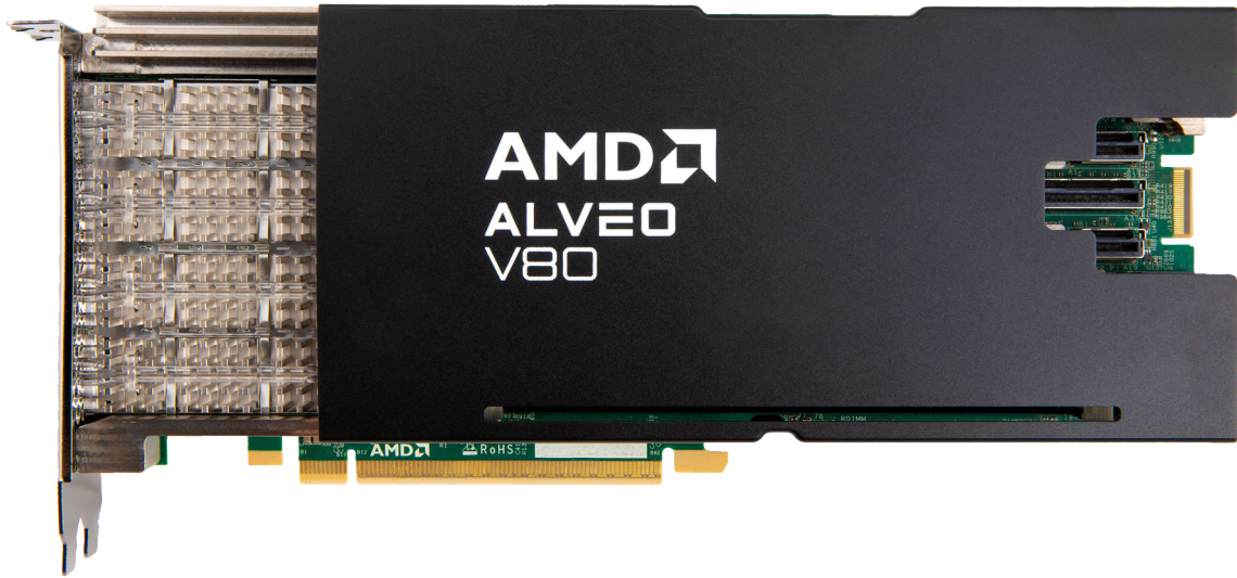
Figure 1: Alveo V80 Card
