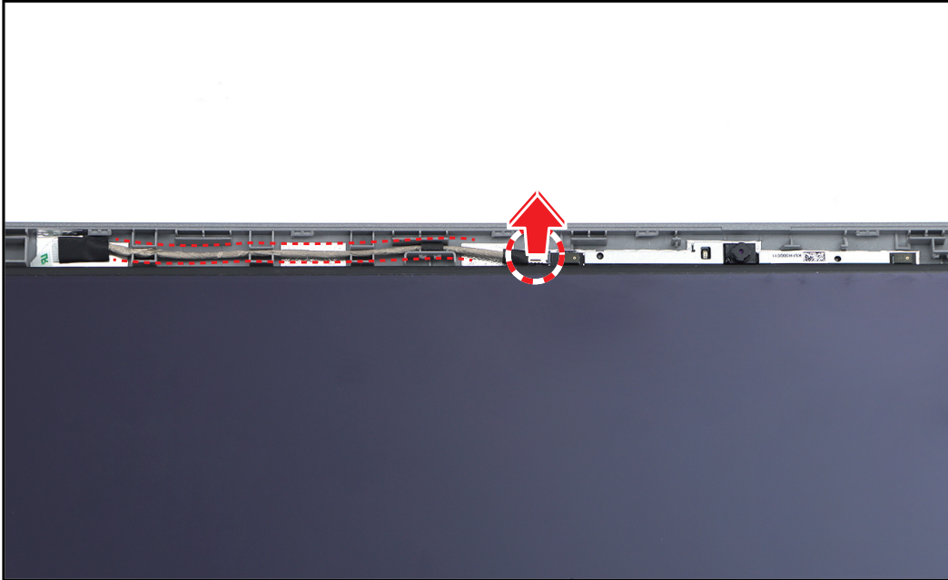
Figure 1-46. Disconnecting and Unrouting the eDP Cable
