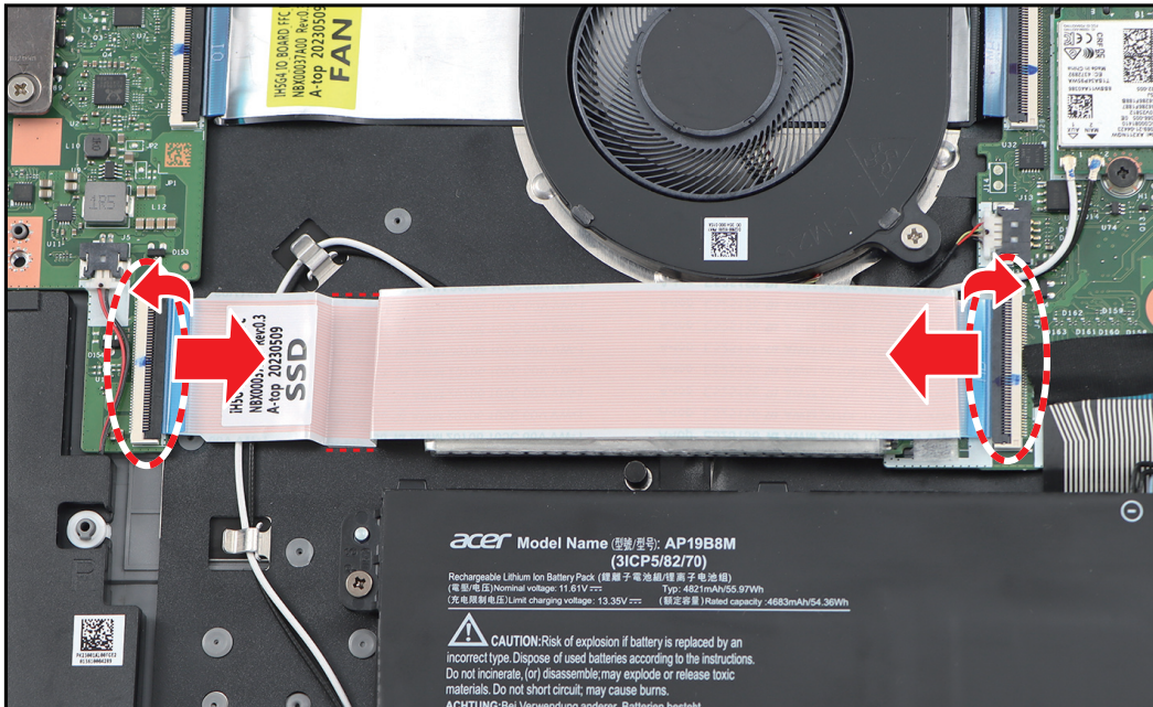
Figure 1-13. Disconnecting and Removing the USB Board FFC
